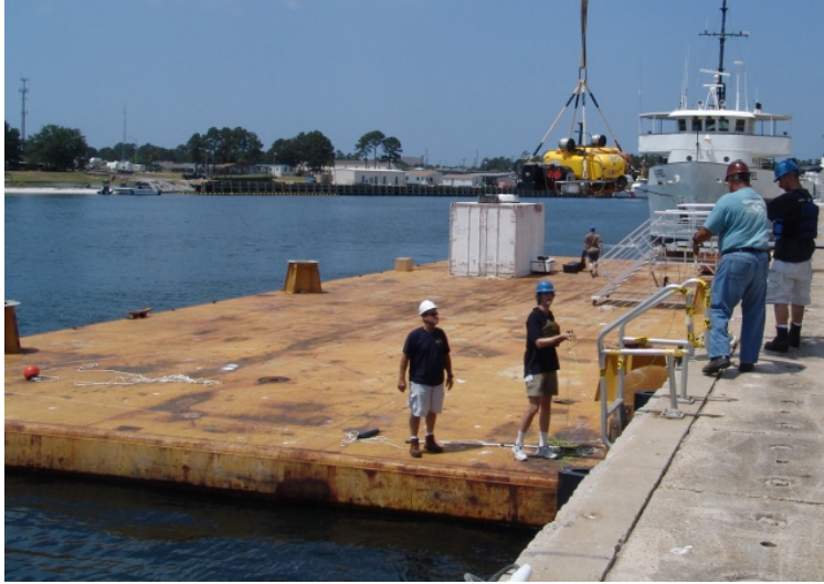
Figure 5-6: The first version of the HAUV being lowered into the water to survey the barge during AUVFest. The barge is 13.4 m from port (side nearest to the pier) to starboard and 36.2 m from bow to stern.
