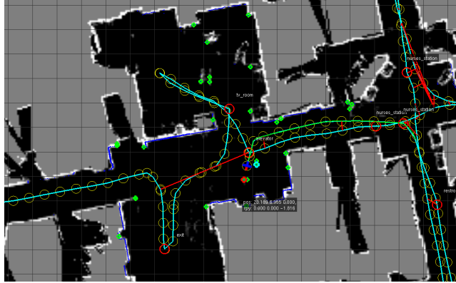
Figure 6-1: SLAM Output: Segments which might have been generated by legs are circled in green.
